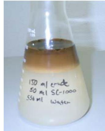
Illustrates the separation of crude oil and water using our plant-based, non-ionic surfactant system: SC-1000
